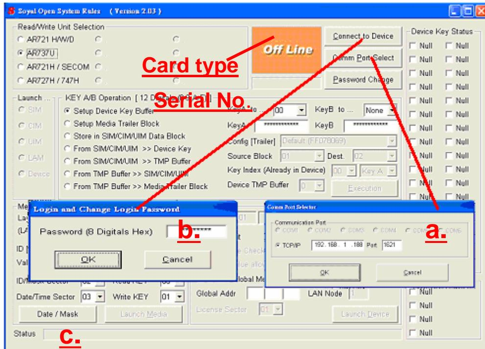
1. Click "Comm Port Select" to select communication type (RS-232, USB or TCP/IP) as shown on [a.](#)
