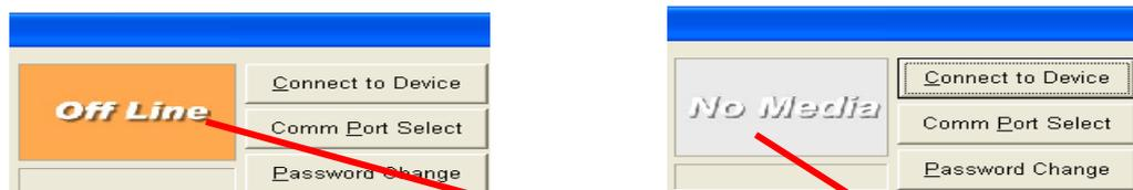
4. When the value of "Card Type" shows from [Off Line](#) to [No Media](#) and gives a beep sound, and the message "[Device Login OK](#)" is given by "Status" column means the programmer is connecting to the PC as shown on [c.](#)
